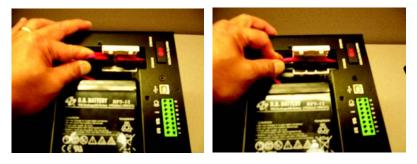
5. To complete the battery installation, close the white connector retainer and reattach the battery door with the three screws (torque of 8.7+/-1.7 lb-in).
