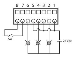
To enable the UPS, close the switch that is connected to the Dry I/O terminals 7 and 8.
