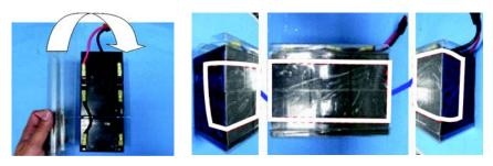
**5.** To connect the batteries to the UPS, insert the batteries into the battery compartment, open the white connector retainer and connect the two cables together as shown in the photo below.
