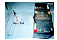
**3.** Connect the red wire of the harness to the positive terminal (top red) and the black wire of the harness to the negative terminal (bottom black). See photo below for details.
