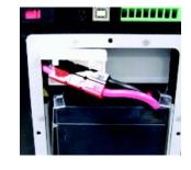
6. To complete the battery installation, close the white connector retainer and reattach the battery door with the three screws (torque of 8.7+/-1.7 lb-in).
